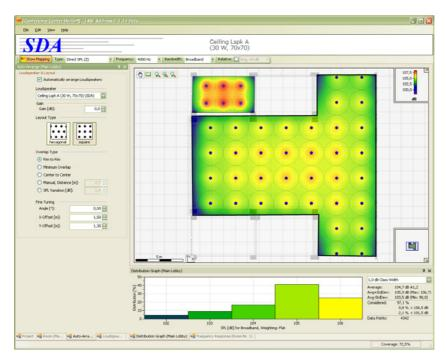
EASE Address makes it easy to draw or import rooms, apply customizable ceiling grids, and view accurate calculations of direct sound coverage patterns.
